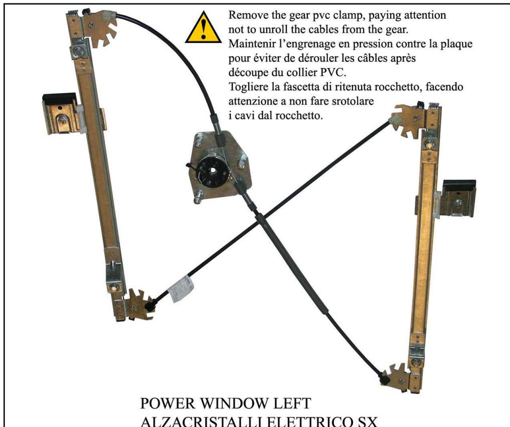
Remove the gear pvc clamp, paying attention not to unroll the cables from the gear.
